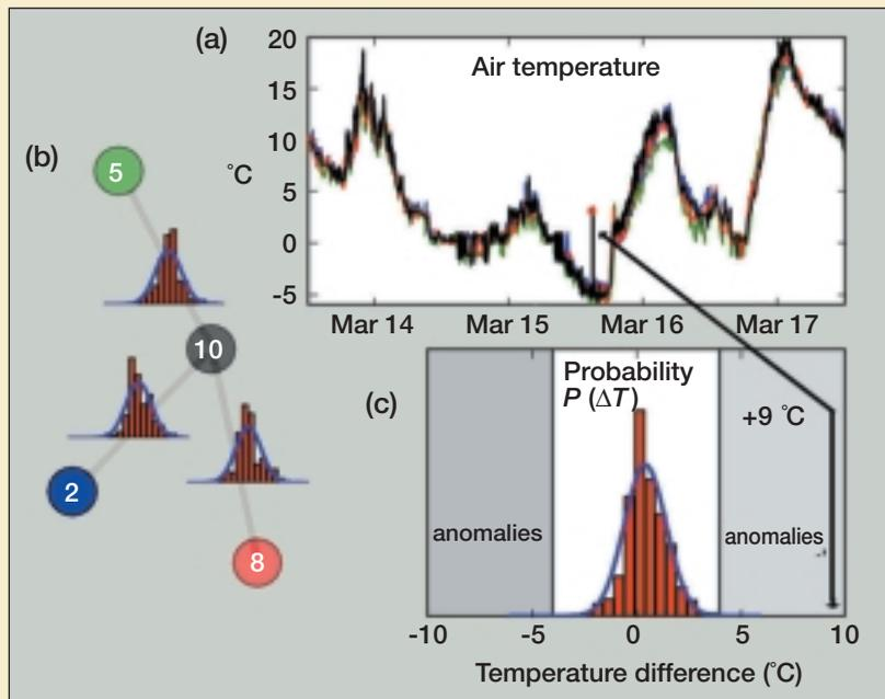
**Figure 4.** A data transmission anomaly (a; red circle) in the air temperature measurements at one of the Sensor Web pods can be identified and eliminated via comparison to the measurements transmitted by nearest-neighbor pods (b). The anomalous reading is identified as an outlier (c) in the distribution of differences between the readings at a pod and those of its neighbors at a predetermined level of statistical confidence (Larkey *et al.* unpublished).
