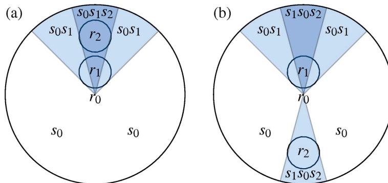
**Figure 3:** Diagram for the two-dimensional example. The source position  $\tau_0$  is fixed in the center and the searchers are disks of radius  $d$ . At each time step, the source emits two particles in opposite directions with a random angle. Each possible emission axis passing through the source corresponds to one of six cases for source and searcher configurations as given in **Tables 1 and 2**.
