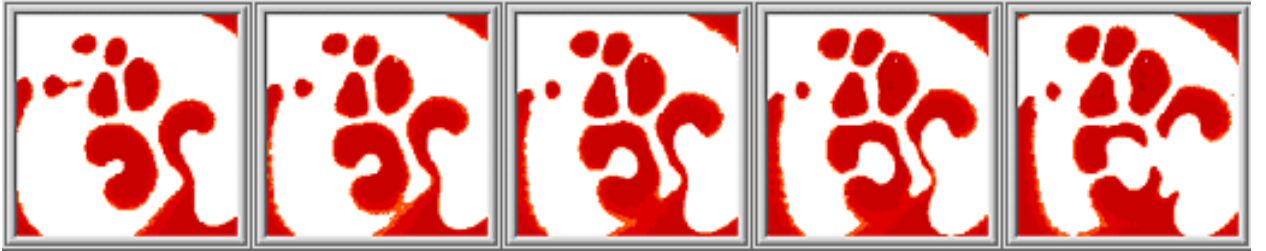
FIG. 6: Patterns in the Ferrocyanide-Iodate-Sulfite reaction show interactions leading to front reversals followed by domain splittings. These images are from experiments performed in the Center for Nonlinear Dynamics at the University of Texas at Austin.
