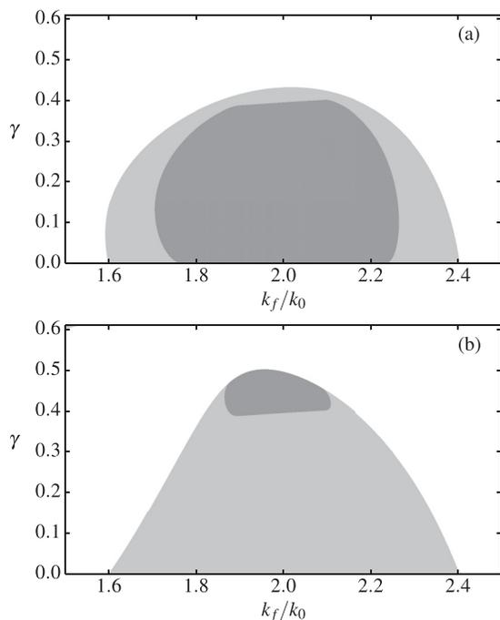
FIG. 3. Existence and stability domains of resonant solutions,  $B_0$ , of Eq. (10) for (a)  $\phi_0 = 0, \pi$  solutions and (b)  $\phi_0 = \pi/2, 3\pi/2$  solutions. The light gray areas indicate the existence domain, while the dark gray area shows the stability region. Parameters:  $a = 10$ ,  $\sigma = 50$ ,  $d = 1$ ,  $w_0 = 0$ , and  $b = 0.185$ .
