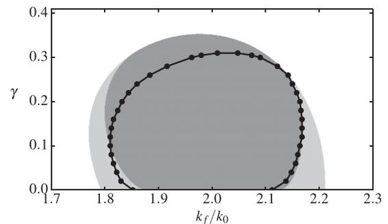
FIG. 2. Existence and stability domains of resonant solutions,  $B_0$ , of Eq. (10) with  $\phi_0 = 0, \pi$ . The light gray areas indicate the existence domain, while the dark gray area shows the stability region. The black curve demarcates the borders of the numerically computed stability region using the LE model (1). Parameters:  $a = 10.5, \sigma = 20, d = 1, w_0 = 0$ , and  $b = 0.25$ . For these parameters, the solutions with  $\phi_0 = \pi/2, 3\pi/2$  are unstable.
