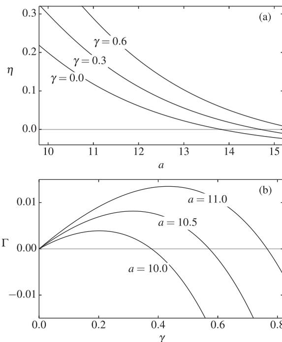
FIG. 1. The coefficients  $\eta$  (a) and  $\Gamma$  (b) of the amplitude equation (10) as functions of the LE model parameters  $a$  and  $\gamma$ . Note that  $\eta$  becomes negative at sufficiently large  $a$  values and that the dependence of  $\Gamma$  on  $\gamma$  is non-monotonic. Parameters:  $k_f/k_T = 1.8$ ,  $d = 1$ ,  $w_0 = 0$ , and  $\sigma = 20$ .
